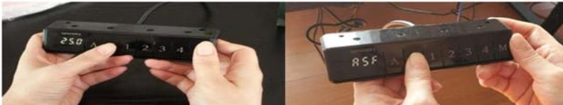
5. Press and hold the **DOWN** button until the desk reaches its lowest position. If the table is already in its lowest position, press and hold the **DOWN** button for 20 seconds.
