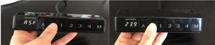
8. Once you see the height of the lowest position displayed on the keypad, release the **DOWN** button. Reset is now complete.
